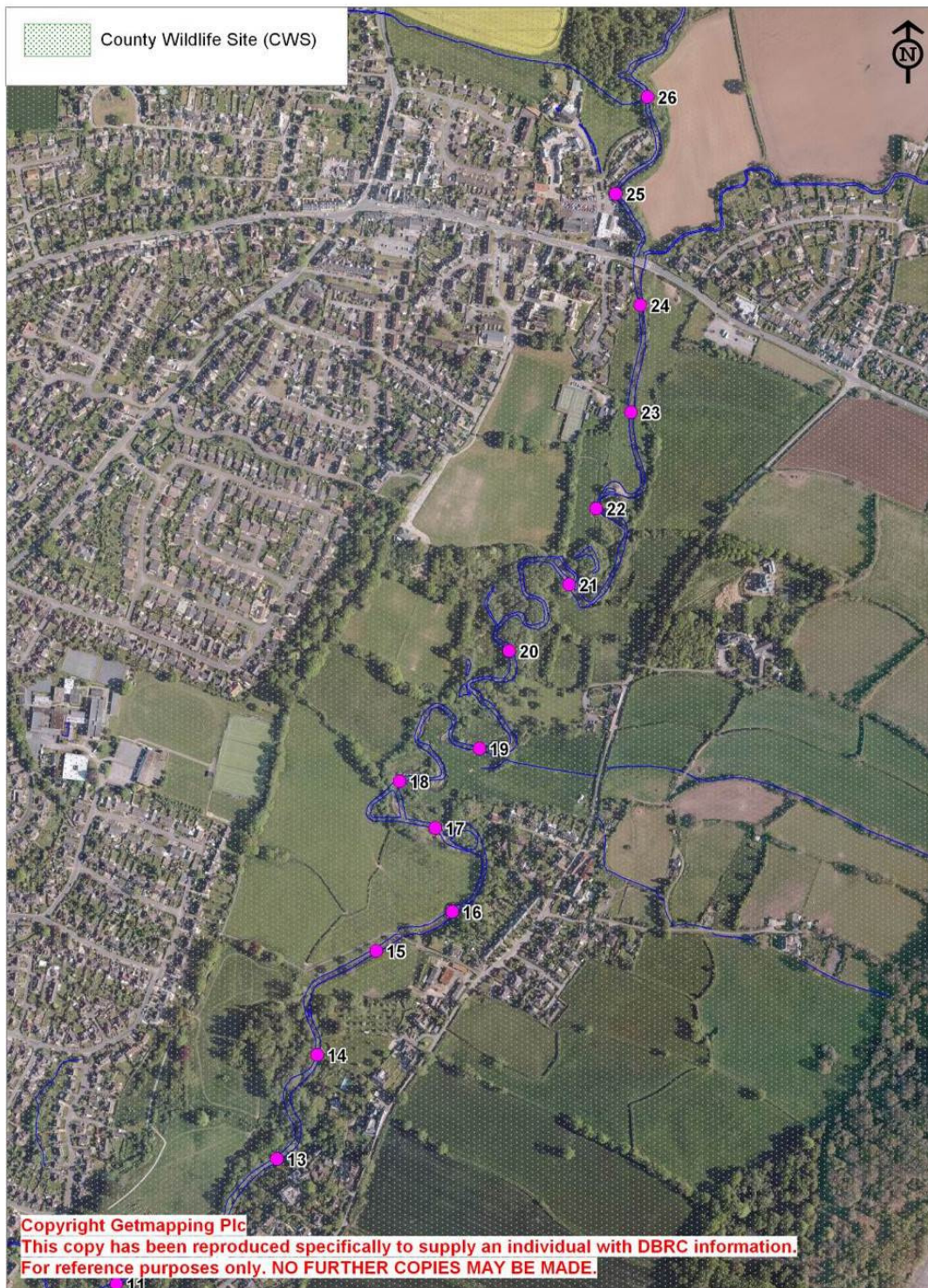
Map 4: The Sid catchment was subdivided into 177 stretches of watercourse for surveying and mapping purposes, each approximately 150-200 metres in length. This map defines the extent of sections 11 to 26.
