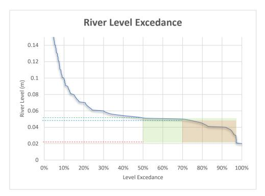
Figure 10 Detailed water level exceedance curve (ID 45216)
